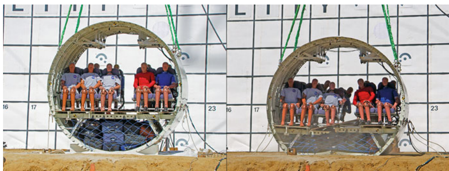
Fig. 1.4 Regional jet fuselage tests at the NASA Langley Research Center Crash Test Facility (Photo Credit: NASA Langley Research Center) [9]
