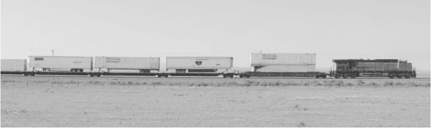
Fig. 2.6 Freight train pulling cars loaded with intermodal shipping containers and truck trailers
