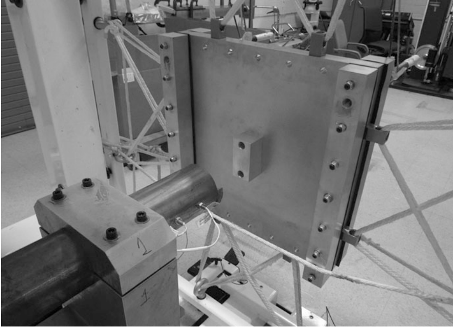
Fig. 9.6 Rear view of a resonant plate shock machine showing impact anvil and gas gun muzzle
