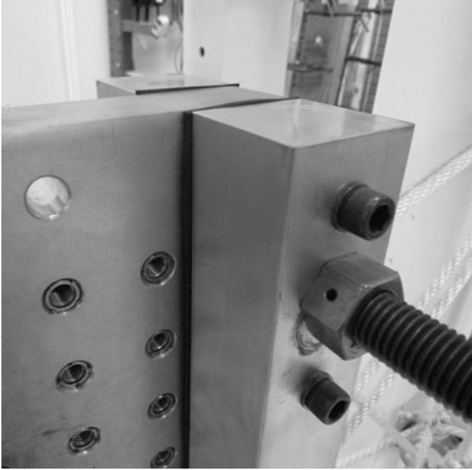
Fig. 9.7 Close-up view of damping bars and damping material attached to a resonant plate
