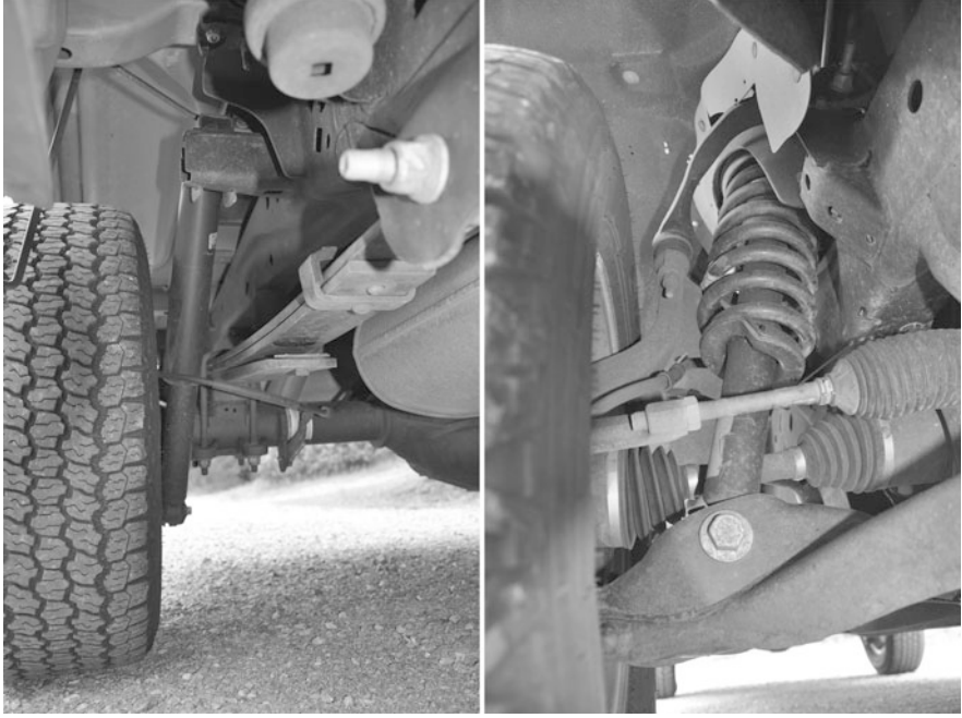
Fig. 2.4 Common vehicle suspension types: leaf springs with shock absorber on left, coil over shock absorber on right
