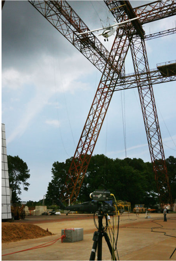
Fig. 1.3 A Cessna 172 suspended in the NASA Langley Research Center Crash Test Facility (Photo Credit: NASA Langley Research Center)
