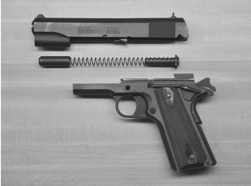
Fig. 2.11 Photograph of a disassembled pistol with the recoiling mass on top, the recoil spring in the center, and the frame beneath
