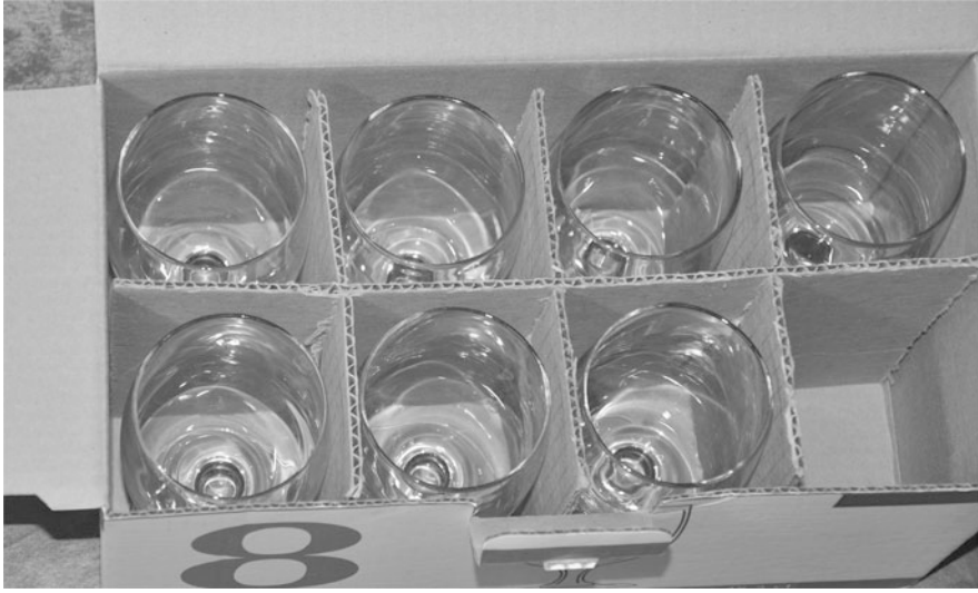
Fig. 2.1 Glass goblets shipped in a cardboard box with dividers to prevent impacts between glasses
