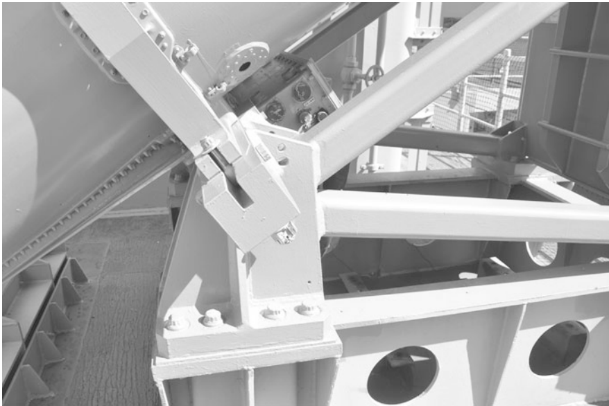
Fig. 7.12 Photograph of one of the mounting feet for an old U.S. Navy Harpoon missile launcher
