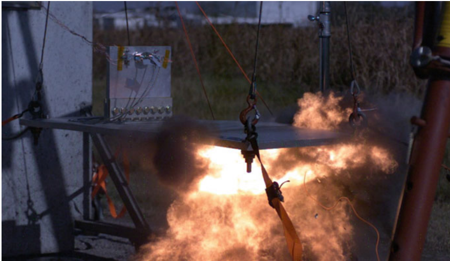
Fig. 2.10 Photograph of a pyrotechnic test of an electronic component (Photo Credit: NASA Johnson Space Center) [3]
